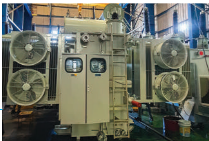
25/35 MVA, 13.8/13.8 KV, 60 Hz Unity Ratio Transformer supplied to Texas, USA.
