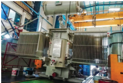
12 MVA, 13.8/12.47 KV 60 Hz Interconnecting Transformer supplied to Texas USA.
