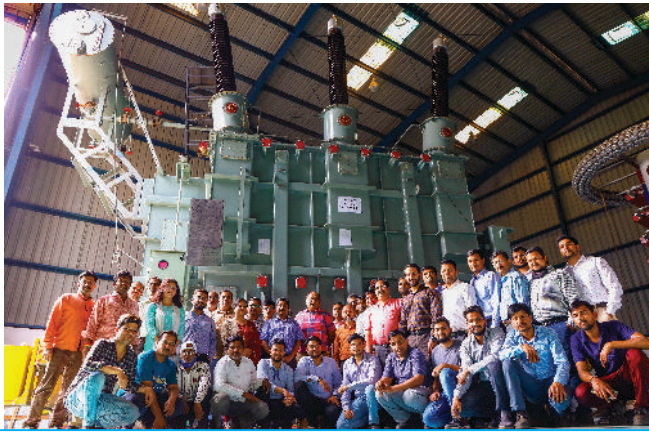
50 MVA, 220 KV Power Transformer
