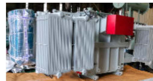
2 MVA 27.6 x 0.6kV Supplied to Canada
