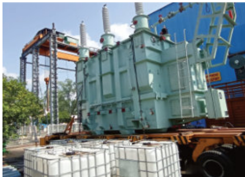
50MVA 132kV at CPRI (STL Lab) for SCT
