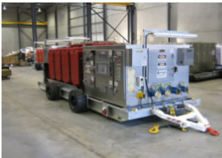
Trailer Mounted Mining Transformer Supplied to Australia
